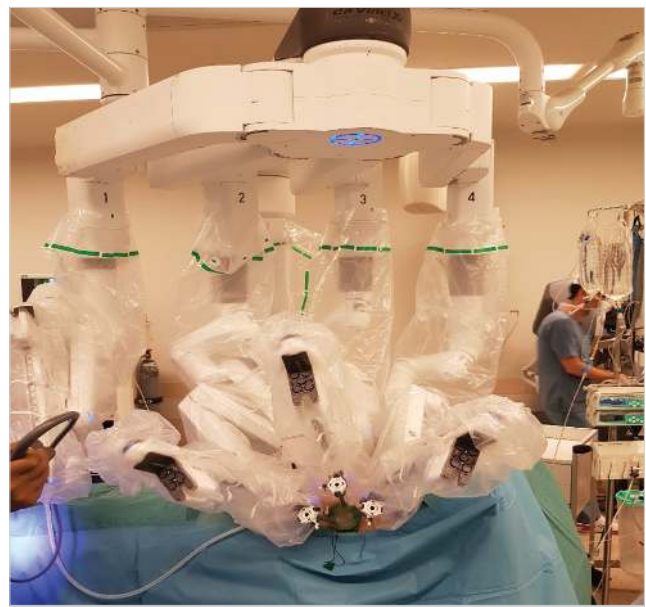
Figure 2. Docking of the Da Vinci Xi Robotic System.
